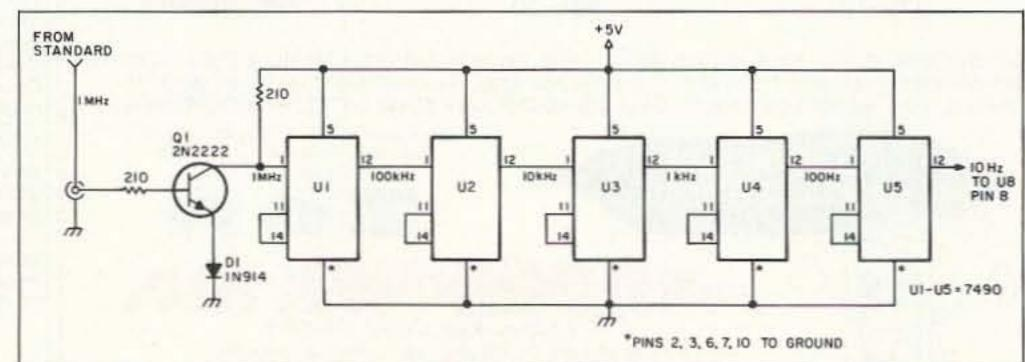
Figure 2. To build this curcuit, you only need five 7490 decade counter/dividers and a piece of perfboard.
